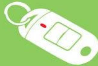
More and more manufacturers are adding **Keyless Ignition Systems** to their vehicles, which usually consist of a device (also known as a key fob or a FOB) carried by the driver, taking over the functions of a traditional metal key.
